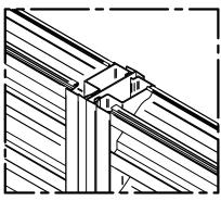
DETAIL C: FRONT VIEW ( CHANNEL FRAME MOUNTING )
